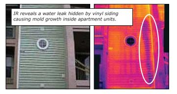
**Energy Efficiency:** IR can detect missing, wet or damaged insulation and identify poorly insulated pipes in buildings, which can increase energy costs.
